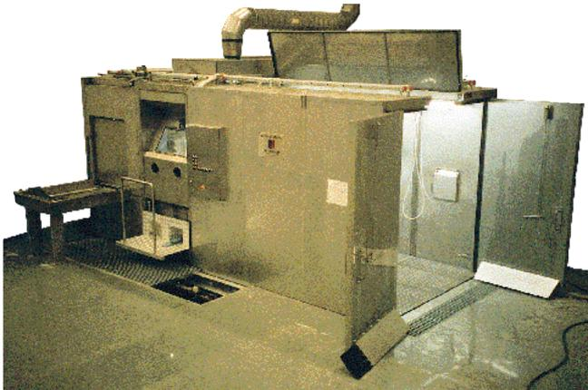
Large wet blasting cabinet DECO-System, a delivery to OKG II in Sweden.
