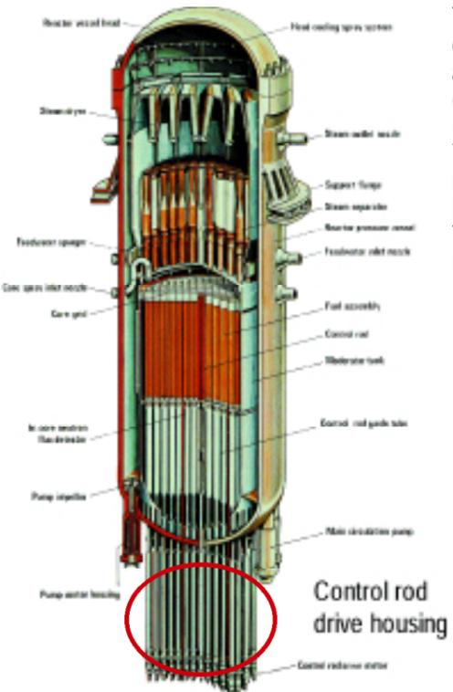
The Control Rods of a BWR reactor are defined as key components as their tasks are to regulate the power during normal operation and to rapidly shut down the reactor to a safe state. To ensure the function of the system, maintenance is performed on each individual CRD at five yearly intervals. The total number of CRD units on a typical BWR reactor is between 120 to 160.
