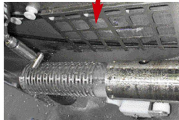
The noise from the nozzles is normally very high (120 dBA) due to very high water velocity. DDT-2000 is efficiently sound insulated which results in a noise level outside the machine of approximately 80 dBA.
