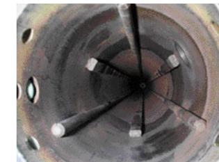
In operation the CRD's are exposed to very high temperatures which means that the surfaces becomes coated with corrosion. The DDT-2000 efficiently removes oxide bound radioactive particles and residual graphite lubricant.
