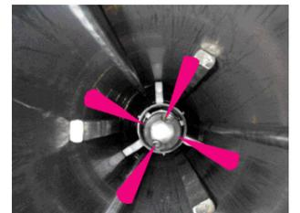
The internal decontamination is performed by four rotating jets. The internal nozzle fits in an internal pipe, diameter of 60 mm and up.
