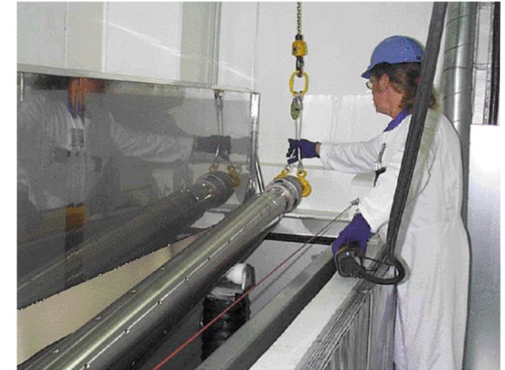
The DDT-2000 is designed for convenient loading and unloading of the CRD parts. Vertical or horizontal handling is possible. Automatic, vertically adjustable supports guarantee the correct location of the CRD parts. A fibre optic system indicates which of the different parts is loaded as well as its location. The DDT-2000 loads automatically the appropriate cleaning program. During external decontamination when the parts are rotating the positioning of the CRD parts is automatically controlled.
